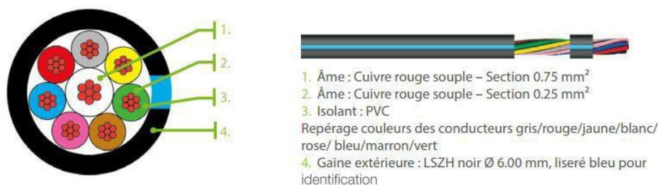
Loop Cable (ref: LC-50/100/150)
