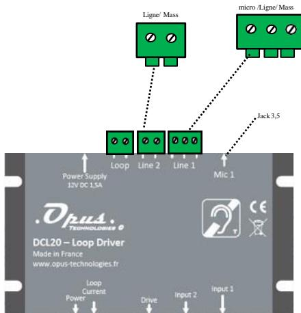
To connect your TV to the DCL20, connect the cable provided in line input 1.
