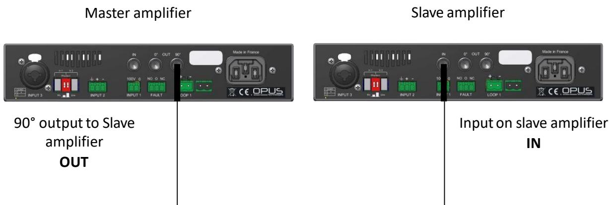
To expand and duplicate an installation or to use a low spill system or high coverage system with the LD Series 1-channel amplifiers:
