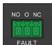
When the amplifier is working properly, the NO/NC relay is activated in the normally closed position: NC.
