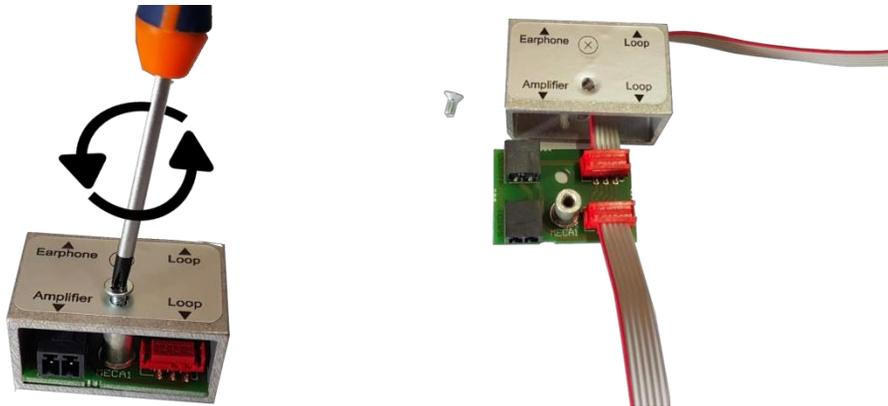
Connect the beginning and the end of the loop cable to the circuit board (red connector).
