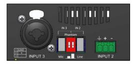
The level of inputs 2 and 3 can be set according to the audio source used.
