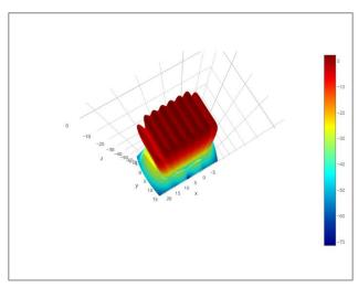
3D view of an ultra-low spill magnetic field
