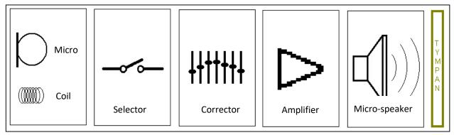
Diagram of operation of a hearing aid with "T" position - Figure 3
