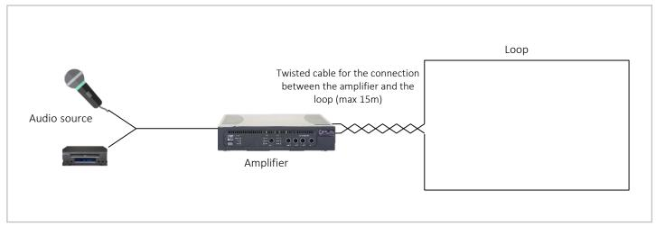
Illustration of a complete magnetic loop system - Figure 13
