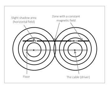
Sectional view of a loop installation in a room - Figure 12
