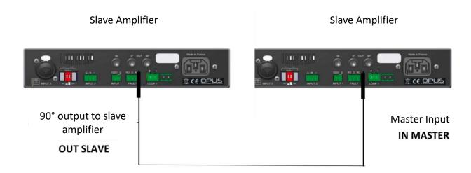
Connect the OUT SLAVE jack of the slave loop amplifier to the MASTER jack of the following slave loop amplifier.
