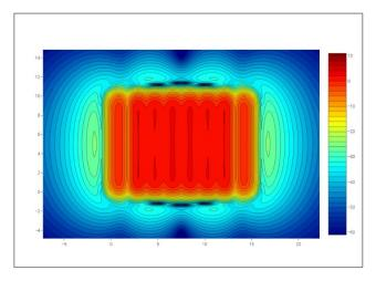
2D view of an ultra-low spill sytem magnetic field
