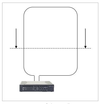
Top view of a loop installation in a room - Figure 11
