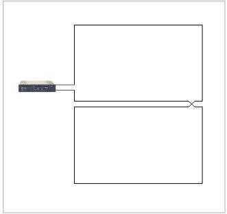
Implantation of a simple loop in a "8" form- Figure 15
